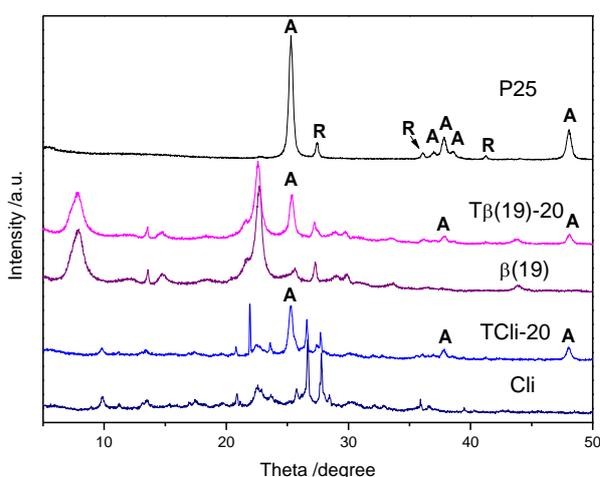
Figure 1. XRPD patterns of P25, starting zeolites (Cli and  $\beta$ (19)) and composite materials (T Cli-20 and T $\beta$ (19)-20). Abbreviations: A-anatase and R-rutile.
