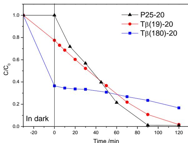
Figure 3. Removal of BPA using:  $C_0= 20 \text{ mgL}^{-1}$  for P25-20 and Tβ(19)-20 and  $C_0= 50 \text{ mgL}^{-1}$  for Tβ(180)-20 (0 min – start of irradiation, C-concentration measured at 225 nm at different irradiation time).
