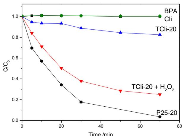
Figure 2. Degradation of BPA ( $C_0= 10 \text{ mgL}^{-1}$ ) using: Cli, P25-20, TCl<sub>i</sub>-20 and TCl<sub>i</sub>-20 with addition of 25  $\mu\text{l}$  H<sub>2</sub>O<sub>2</sub> (0 min – start of irradiation, C-concentration measured at 225 nm at different irradiation time).
