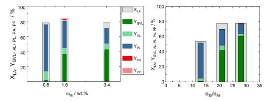
Figure 2. LA conversion (X<sub>LA</sub>), yield (Y) of products (GVL, AL, PL, PA and PP) over the bifunctional catalysts *x*-ZSM-5-21 with  $x = \omega_{Ni} = 0.8$ , 1.6 and 3.4 wt.% (left) or 3.4 wt.% Ni supported on ZSM-5-*y* with  $y = n_{Si}/n_{A1} = 13$ , 21 and 28 (right). Reaction conditions:  $m_{cat} = 100$  mg,  $Q_{H_2} = 30$  ml min<sup>-1</sup>,  $c_{LA} = 1$  wt.-%,  $Q_{LA} = 0.03$  g min<sup>-1</sup>, 250 °C, 4 h.
