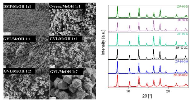
Figure 1. Left - SEM images of ZIF-90 prepared with different solvent ratios; Right - XRD patterns of synthesized ZIF-90.
