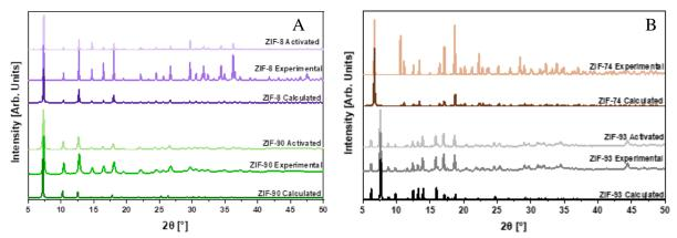
Figure 1. X-ray diffraction patterns of as-synthesized and activated ZIFs. Calculated patterns are also shown. A: ZIF-8 (purple) and ZIF-90 (green). B: ZIF-74 (brown) and ZIF-93 (black/grey).
