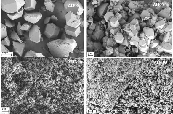
Figure 2. SEM images of as-synthesized ZIF-8, ZIF-74, ZIF-90 and ZIF-93.
