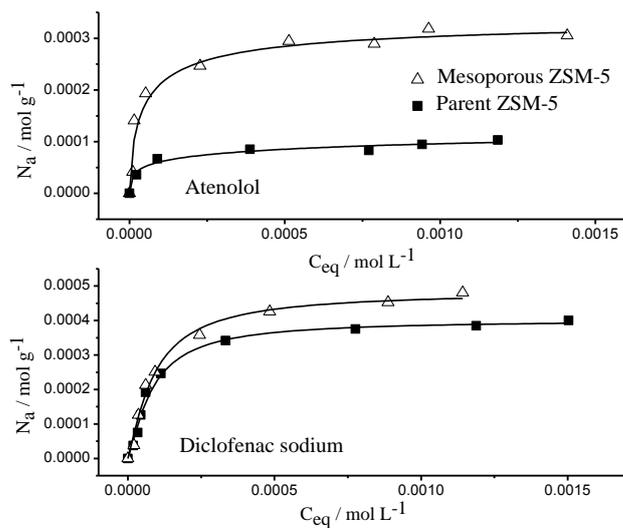
Figure 3. Isotherms of diclofenac-Na and atenolol adsorption on parent and mesoporous HZSM-5 zeolite.
