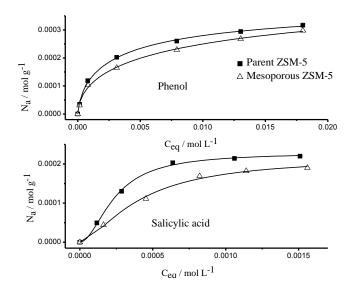
Figure 2. Isotherms of salicylic acid and phenol adsorption on parent and mesoporous HZSM-5 zeolite.
