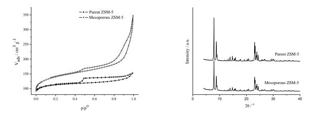
Figure 1. Textural properties (left) and XRD patterns (right) of parent and mesoporous HZSM-5 zeolite.
