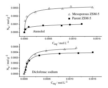
Figure 3. Isotherms of diclofenac-Na and atenolol adsorption on parent and mesoporous HZSM-5 zeolite.
